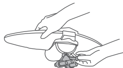
Install the counterweight support secondly
